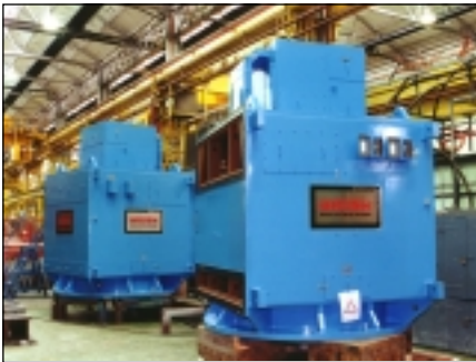
The first two vertical-shaft, water-cooled stern-thruster motors.
