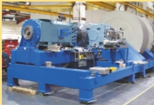
The photographs show the large rear axle rollers being fitted with their shaft bearing arrangements and the complete rear axle assembly during pre-delivery factory tests.
