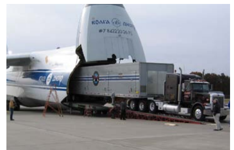
Above: P&W FT8 Mobile Pac generator set being loaded into an Antonov heavy haul aircraft for transportation
