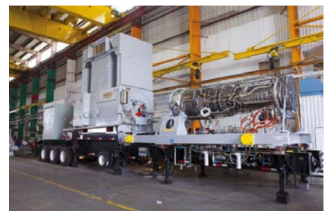
Above: BRUSH BDAX 62-170ER mounted on the GE TM2500 trailer during assembly operations in Houston
