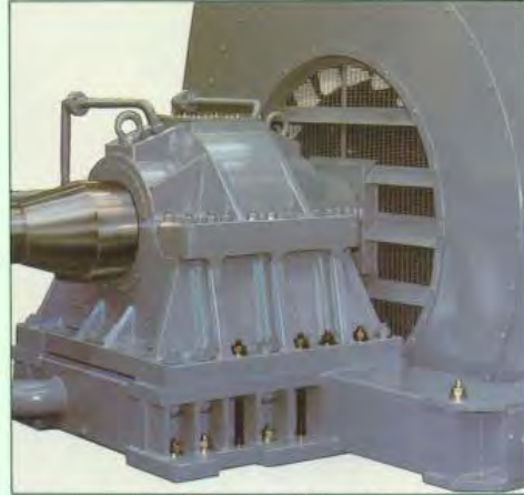
Fig. 22. A special marine type thrust block bearing to take high axial thrust was fitted to this 5.2 MW generator.
