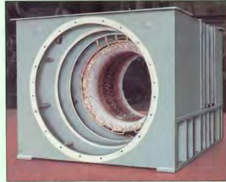
Fig. 14 Stator frame with completed winding. The frame also supports the magnet of the inboard mounted exciter.
