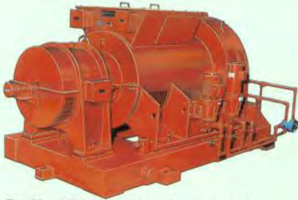
Fig. 30. 300 kW, 1200 rev/min (overspeed 1310 rev/min) 415 V, 3 ph, 50 Hz generator for the South of Scotland Electricity Board's Loch Braden Site. Supplied through Gilbert, Gilkes and Gordon.
