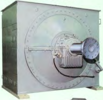
Fig. 32. 1.976 MW, 514 rev/min (overspeed 1000 rev/min) 4160 V, 3 ph, 60 Hz generator for Dillon Dam, U.S.A. For other details see caption Fig. 9.
