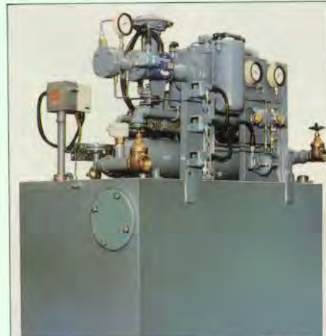
Fig. 27. Complete lubrication module supplied for a 5.2 MW generator.
