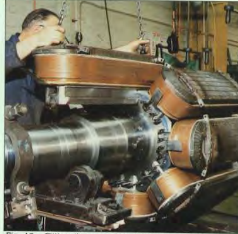
Fig. 19. Fitting the completed pole to the hub.
