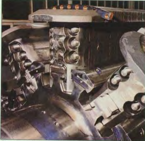
Fig. 18. Detail of inverted double T fitting of the pole bricks to the hub, and the cast steel pole end-plates giving support to the ends of the rotor coils particularly during overspeeds.
