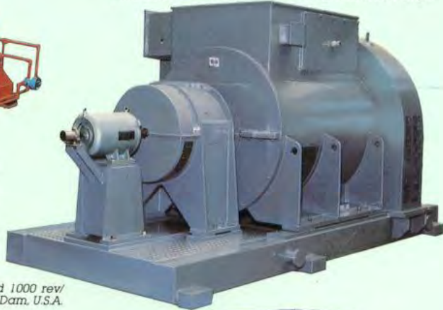
Fig. 31. One of two 830 kW, 1200 rev/min (overspeed 2052 rev/min), 4160 V, 3 ph, 60 Hz generators for Quiroz, Peru. Supplied through Balfour Beatty and Weir Pumps.
