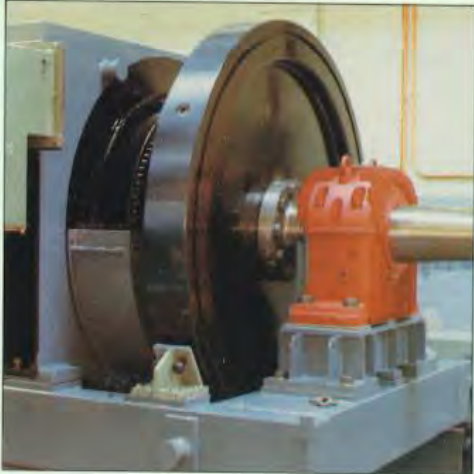
Fig. 21. Sub-assembly in the factory showing flywheel cover removed from a 686kW hydro-generator for installation in Peru.
