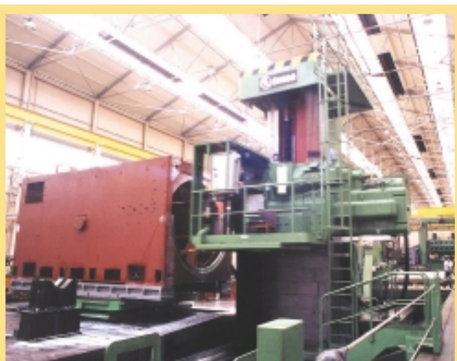
New floor borer machining a DAX turbo generator stator frame
