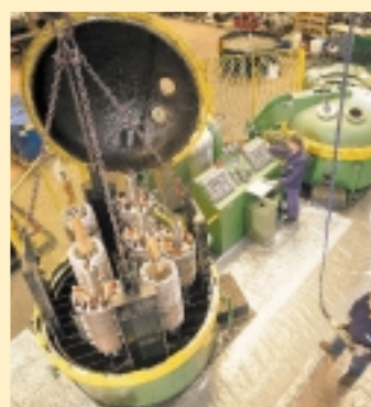
Marelli's VPI plant in operation
