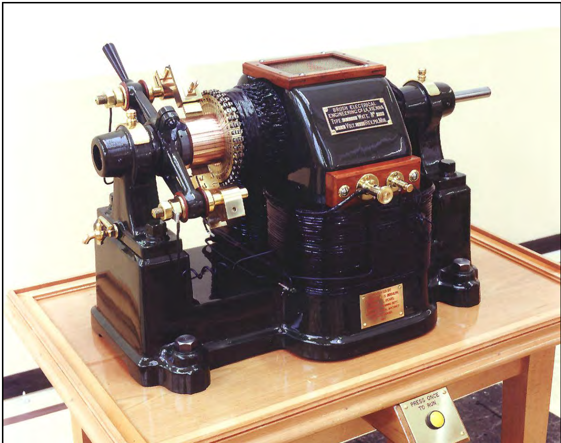
In 1992, Brush Apprentices renovated and rebuilt this 1880 Brush "Vienna" dynamo for company display.
