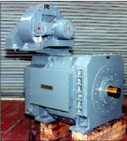
One of the eight anchor windlass motors
