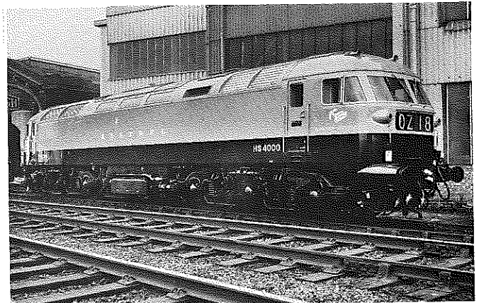
'Kestrel' 4000 H.P. Diesel Electric Locomotive for freight and passenger service.
