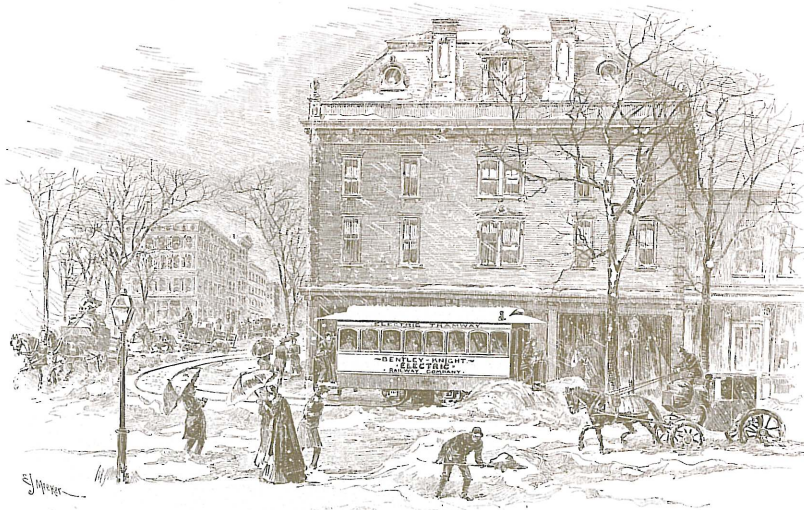
A Bentley-Knight trolley, powered by contact with an electric conduit between the tracks.
