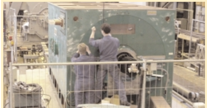
DAX generator being assembled for test
