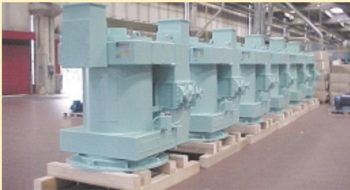
Vertical IP55 motors with air-water coolers at the Marelli factory.
