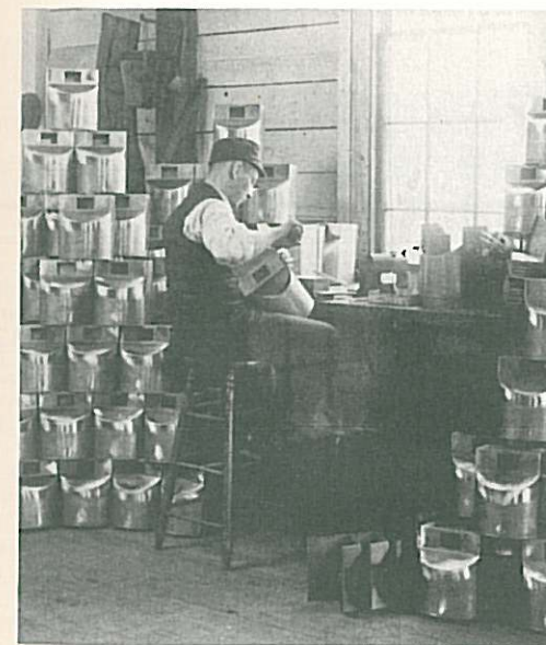
Soldering wattmeter housings at Lynn, Massachusetts.
